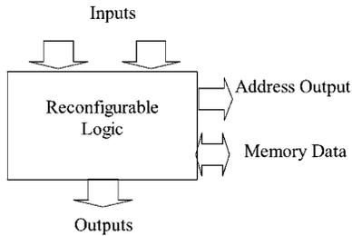
Fig. 5. A reconfigurable functional unit with memory access.
