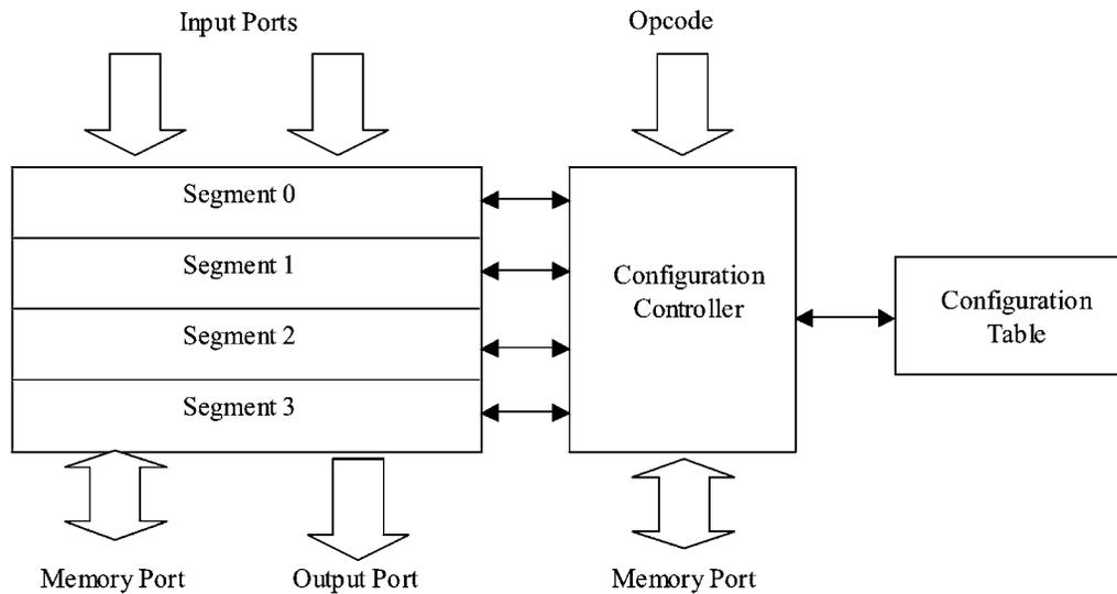
Fig. 9. Detailed view of a reconfigurable functional unit.
